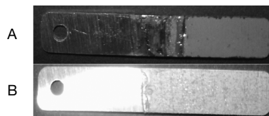
Fig. 9. The anticorrosive effect of Zn-HDTMP films on carbon steel. The upper specimen is the “control” (A), no inhibitor present. Corrosion inhibition in the lower specimen (B) by a 1 mM Zn^{2+} /HDTMP synergistic combination is dramatically demonstrated.
